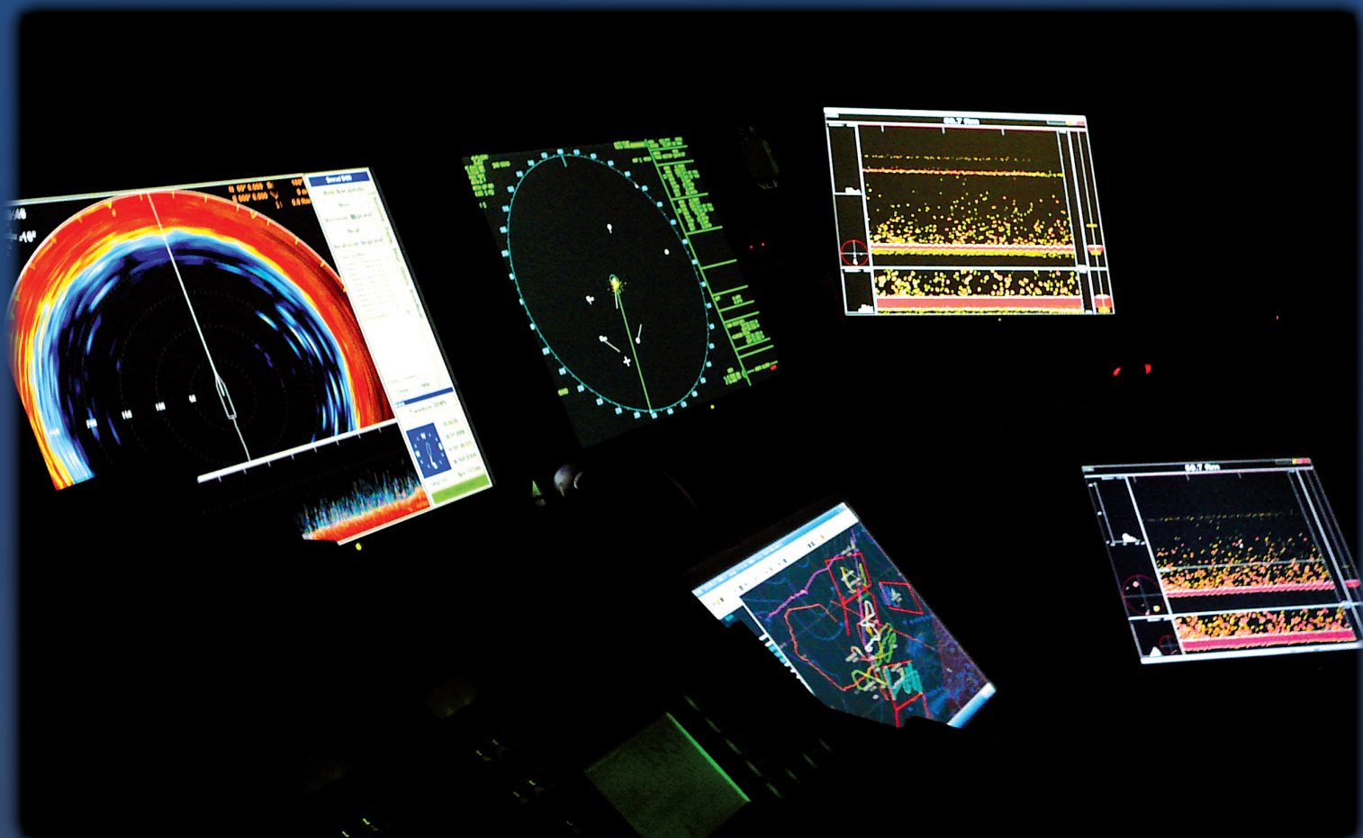
Picture from a bridge during Pollock fishery in Alaska. The picture shows an evening/night time situation when the Pollock is dispersed into “Salt and Pepper”. The SX90 Sonar to the far left and the ES Echosounders to the far right.
